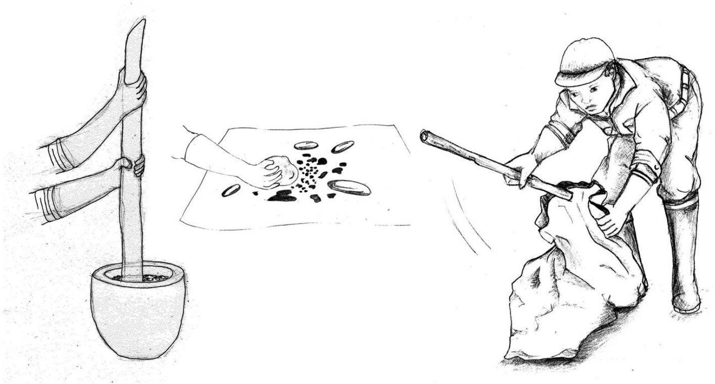
Figure 2-8: Crush the carbonised material into a coarse powder.
