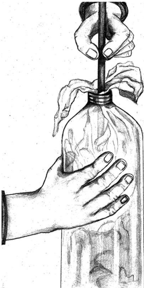
Figure 9-1: Make an ecobrick by stuffing plastic waste inside a bottle.
