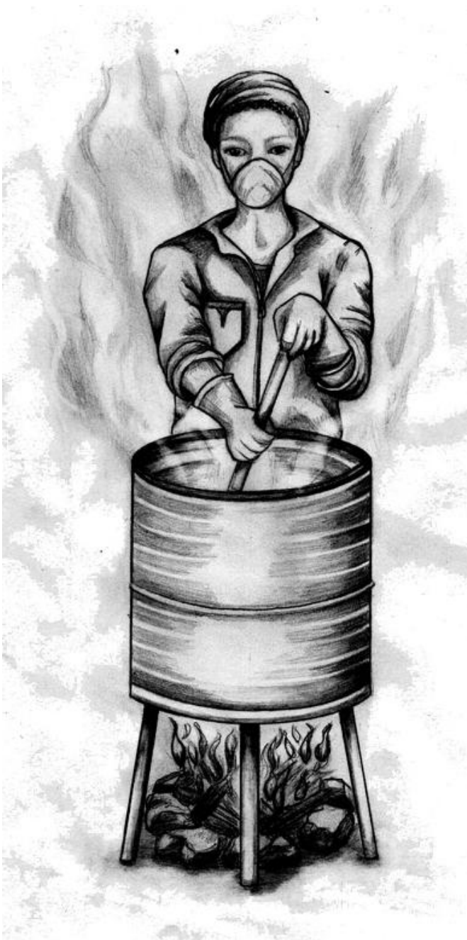
Figure 8-6: Keep mixing the melting plastic until it is a black liquid with no lumps.
