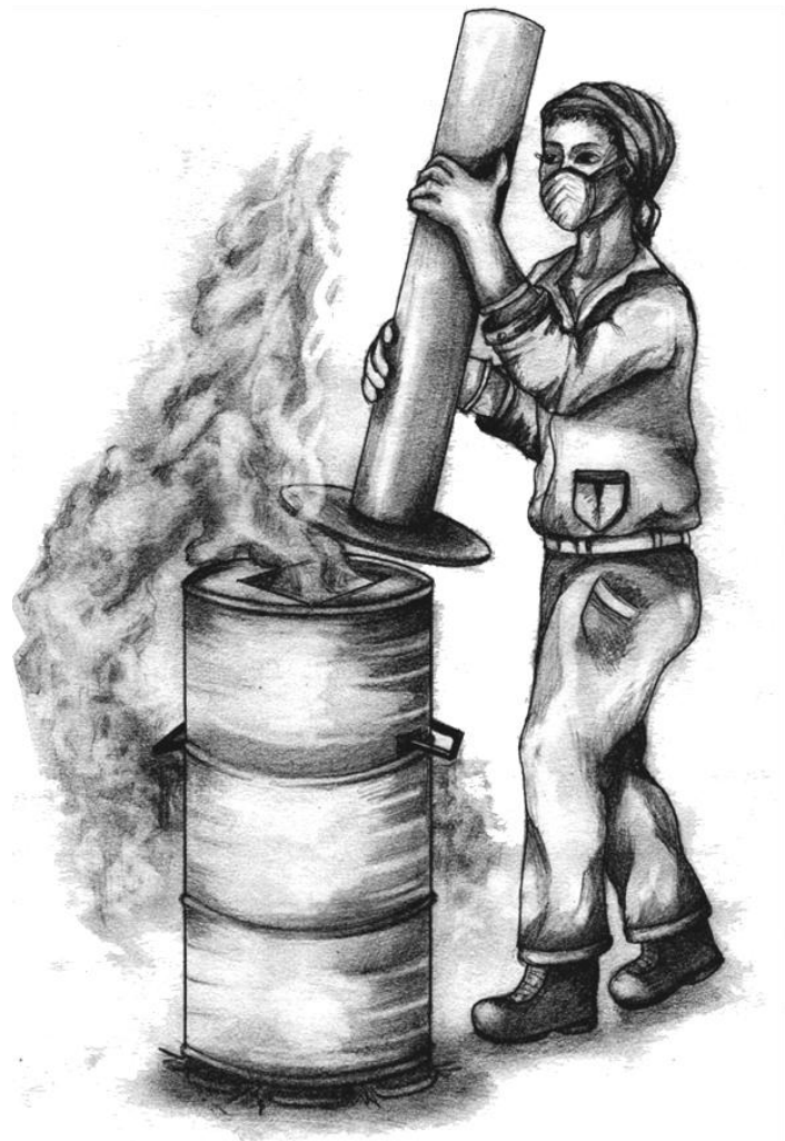
Figure 2-6: Allow the material to carbonise but do not let it burn completely. A chimney is useful to direct the smoke away.
