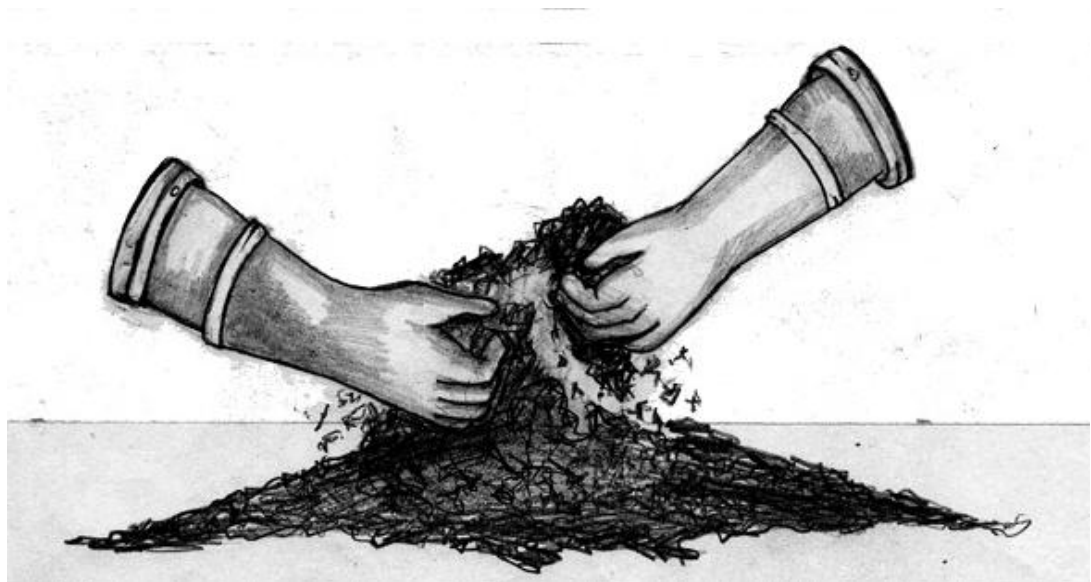
Figure 2-10: Make a mound of powdered char, scoop out a hollow and mix in the binder (like making bread).
